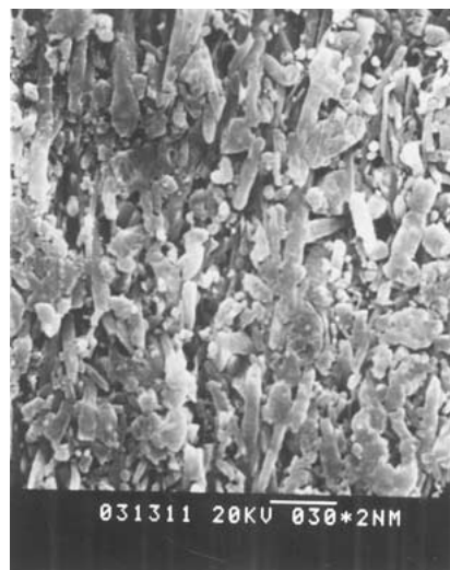
Figure 7 SEM microstructure of samples after creep at 1000^\circ\text{C} .
